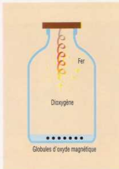
FIGURE 4 Combustion du fer.
